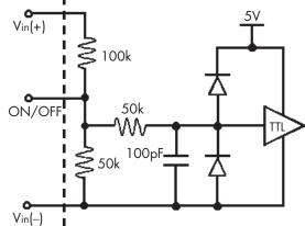
Figure B: Internal ON/OFF pin circuitry (detail)
