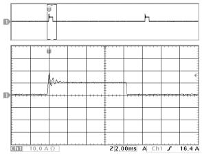
Figure 17: Load current (10A/div) as a function of time when the converter attempts to turn on into a 10 m $\Omega$  short circuit. Top trace (40ms/div) is an expansion of the on-time portion of the bottom trace.
