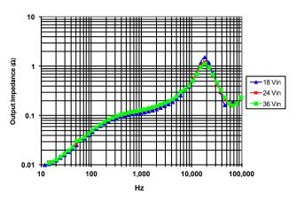
Figure 18: Magnitude of incremental output impedance  $(Z_{out} = v_{oul}/i_{out})$  for minimum, nominal, and maximum input voltage at full rated power.
