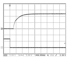
Figure 9: Turn-on transient at full load (resistive load) (4 ms/div). Ch 1: Vout (5V/div). Ch 2: ON/OFF input (5V/div)
