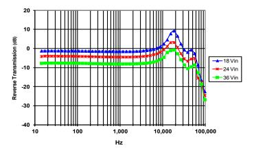
Figure 20: Magnitude of incremental reverse transmission  $(RT = i_{in}/i_{out})$  for minimum, nominal, and maximum input voltage at full rated power.
