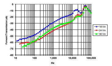
Figure 19: Magnitude of incremental forward transmission  $(FT = v_{out}/v_{in})$  for minimum, nominal, and maximum input voltage at full rated power.
