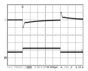
Figure 12: Output voltage response to step-change in load current  $(50\%-75\%-50\% \text{ of } Iout(max): dI/dt = 5A/\mu s).$
