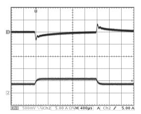
Figure 11: Output voltage response to step-change in load current  $(50\%-75\%-50\% \text{ of } Iout(max); dI/dt = 0.1A/\mu s).$
