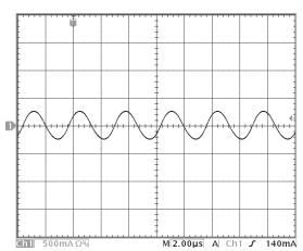
Figure 14: Input Terminal Ripple Current,  $i_c$ , at full rated output current and nominal input voltage with 3.3 $\mu$ H source impedance and  $100\mu$ F electrolytic capacitor (500 mA/div). See Figure 13
