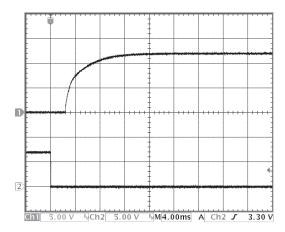
Figure 10: Turn-on transient at zero load (4 ms/div). Ch 1: Vout (5V/div) Ch 2: ON/OFF input (5V/div)
