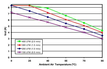
Figure 7: Maximum output power derating curves vs. ambient air temperature for airflow rates of 100 LFM through 400 LFM with air flowing from pin 1 to pin 3 (nominal input voltage).
