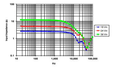
Figure 21: Magnitude of incremental input impedance  $(Z_{in} = v_{in}/i_{in})$  for minimum, nominal, and maximum input voltage at full rated power.
