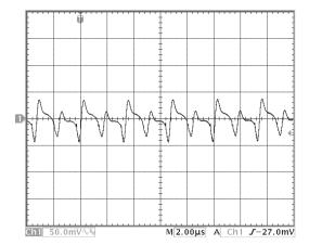
Figure 16: Output voltage ripple at nominal input voltage and rated load current (50 mV/div). Load capacitance:  $1\mu F$  ceramic capacitor and  $10\mu F$  tantalum capacitor. Bandwidth: 20 MHz. See Figure 13.
